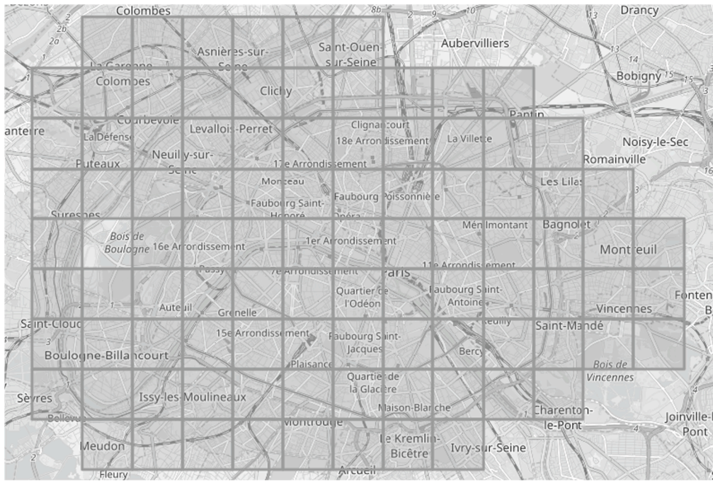
Fig. 1. Gridification for delivery locations in Paris with a pixel size of 1 km 2 .
